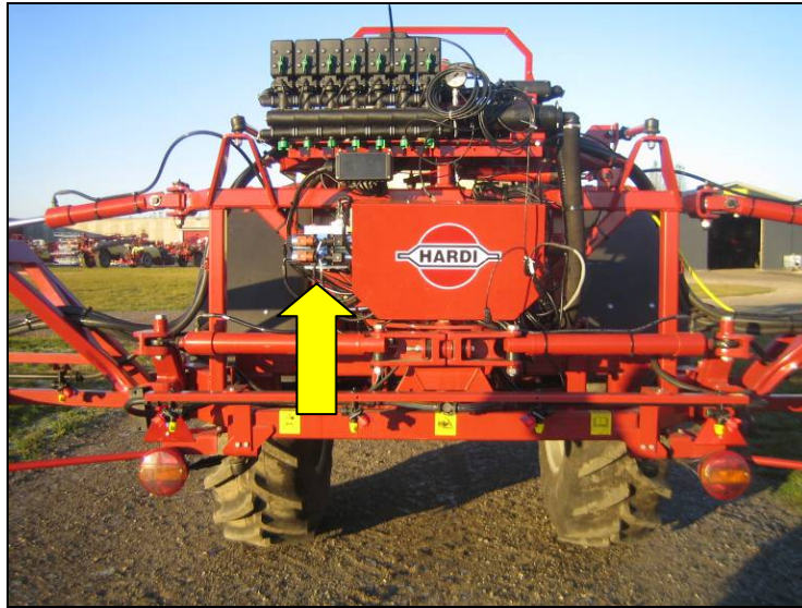
Figure 25: Valve Block Mounting Location on LPZ
