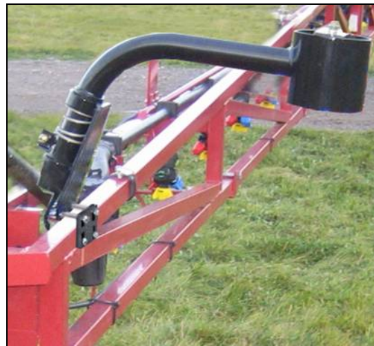
Figure 13: Suggested Bracket Mounting Location on LPZ Boom
