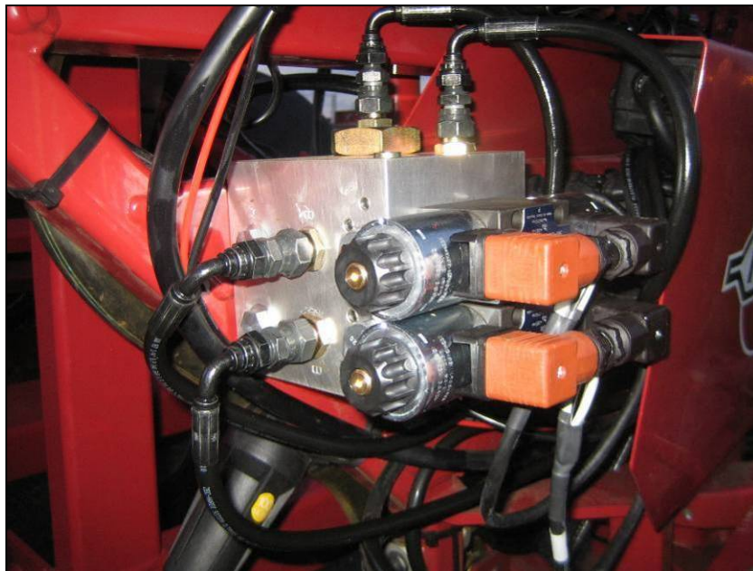
Figure 26: Valve Block Mounted on LPZ
