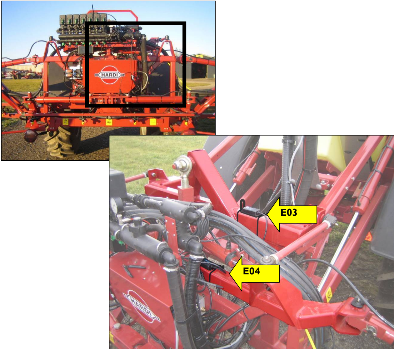
Figure 20: Boom Roll Sensor Mounting (viewed from rear of sprayer)
