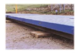
NORAC's portable truck scales require some simple levelling with timbers at each load cell location and at each end of the scale.
